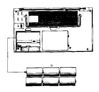
Insert the bottom projections on the edge of the battery compartment cover inside the lower edge of the compartment opening. Lower the cover, and snap the top latch down until it clicks closed.
